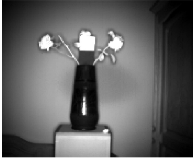
Fig. 4. A line shape region of the cylindrical vase surface (specular) reflects more light than the neighborhood region. At the top of the vase we placed a half white and half black sheet of paper.
